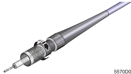
Figure 40 Screwing on the basic unit (with the example of an F-SMA connector)
