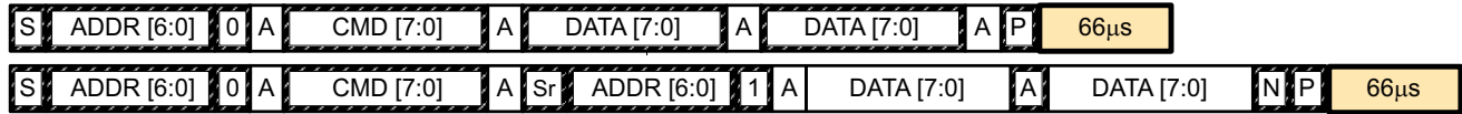
Waiting time inserted between incremental 2-byte write packet for a subcommand and reading results (acceptable for f_{\text{scl}} \leq 100 \text{ kHz} )
