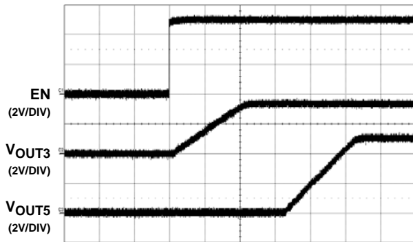
FIGURE 23. DELAYED START WAVEFORMS (EN5 = REF)
