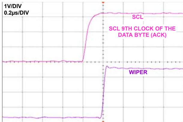
FIGURE 21. WIPER LARGE SIGNAL SETTLING TIME
