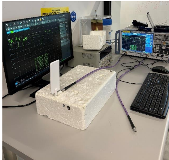
VNA Set up Bent in Free Space
