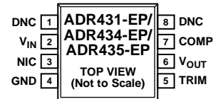
Figure 1. 8-Lead SOIC_N (R-8)
