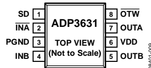
Figure 9. ADP3631 Pin Configuration
