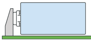
To Mount Battery "On" PC Board Use Cat. No. 593 and Cat. No. 594
