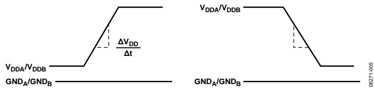
Figure 14. Transient Immunity Waveforms—Output Supplies
