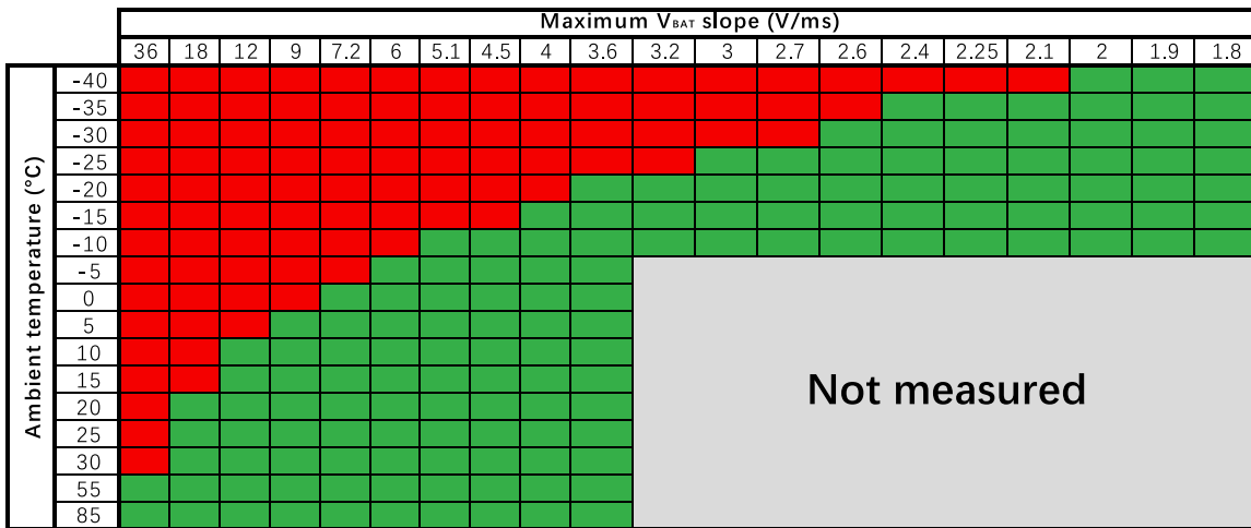
Fig 12. Maximum V_{BAT} slope vs temperature
