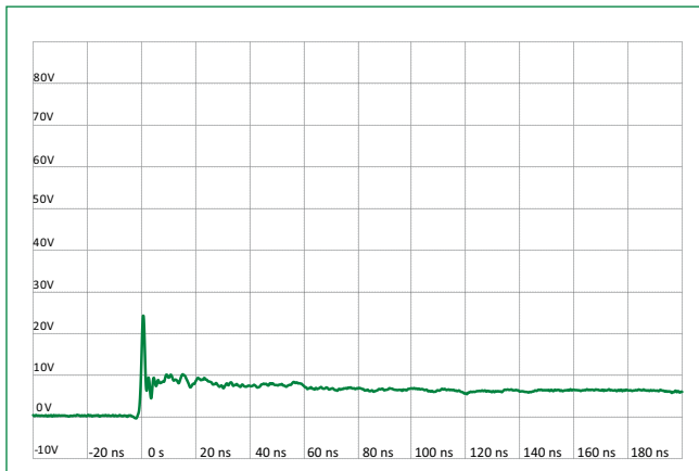
IEC 61000-4-2 +8 kV Contact ESD Clamping Voltage
