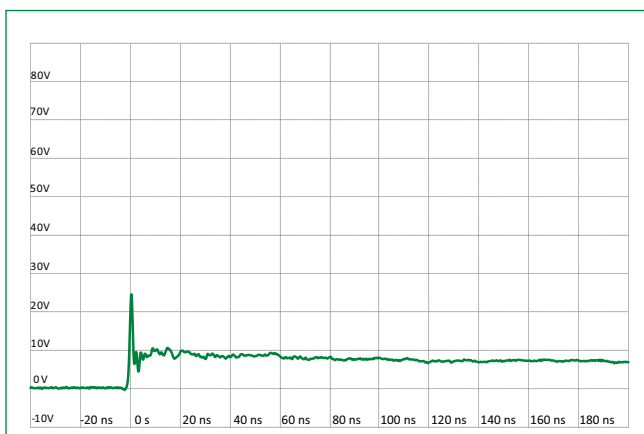
ISO10605 Contact Discharge Plot at +8 kV
