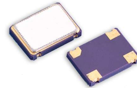
Part Dimensions: 7.0 × 5.0 × 1.8mm • 171.497mg
