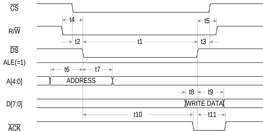
Figure-36 Non-Multiplexed Motorola Mode Write Timing
