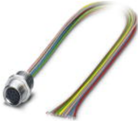
Sensor/actuator flush-type socket, 8-pos., M8, front/screw mounting with M10 fastening thread, with 0.5 m TPE litz wire, 8 x 0.14 mm 2
