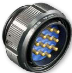
Glenair's "21-12" insert arrangement with 12 size 12 power pins for 23 amp current rating.
