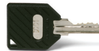
Key Code: A126 4 Tumbler Part No. (One Key) 1159112602 Black Material: Brass Finish: Nickel plate 6/6 Nylon insert molded head
