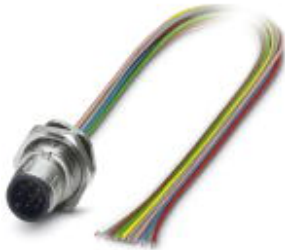
Sensor/actuator flush-type connector, 8-pos., M12-SPEEDCON, rear/screw mounting with Pg9 thread, with 0.5 m TPE litz wire, 8 x 0.25 mm 2
