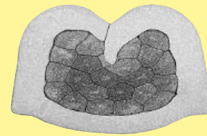
B shape cross section stamped contact
