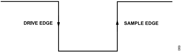
Figure 66. SPI Mode 3, SCLK Edges
