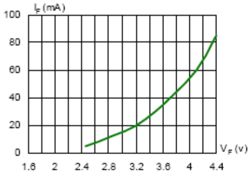
Fig.1 Forward Current vs. Forward Voltage
