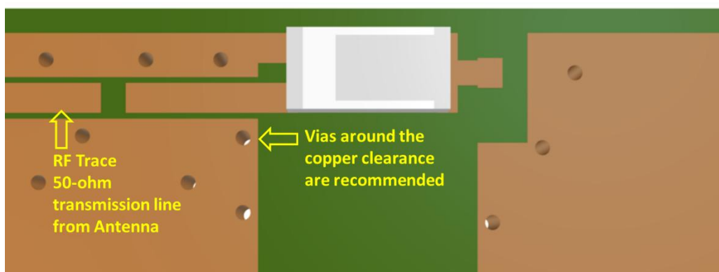
WLA.01 antenna mounted on a PCB, showing transmission line and integration notes.
