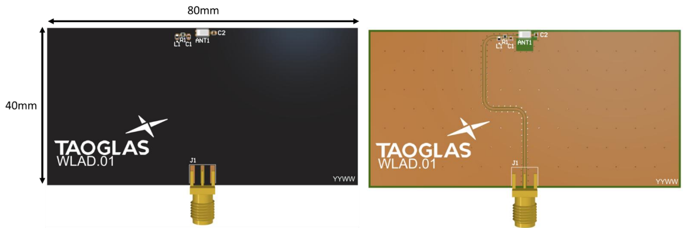
Top Side (WLA.01 placement on 80x40mm PCB)
