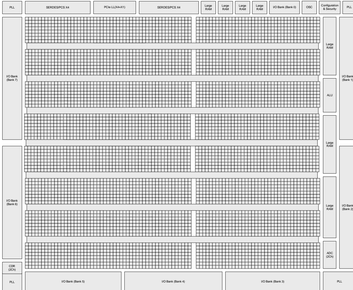
Figure 2.2. Simplified Block Diagram, LFCPNX-100 Device (Top Level)
