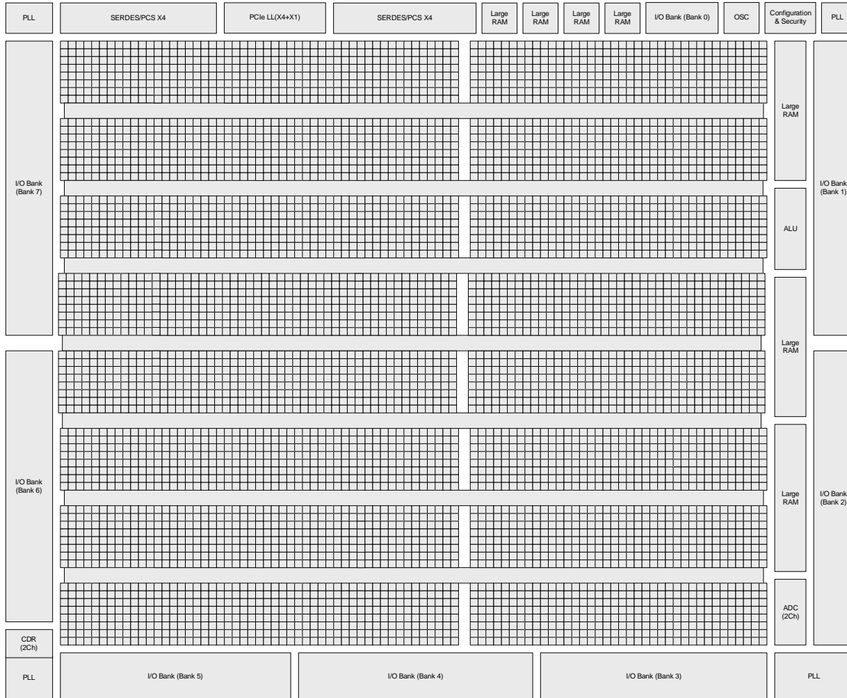
Figure 2.2. Simplified Block Diagram, LFCPNX-100 Device (Top Level)
