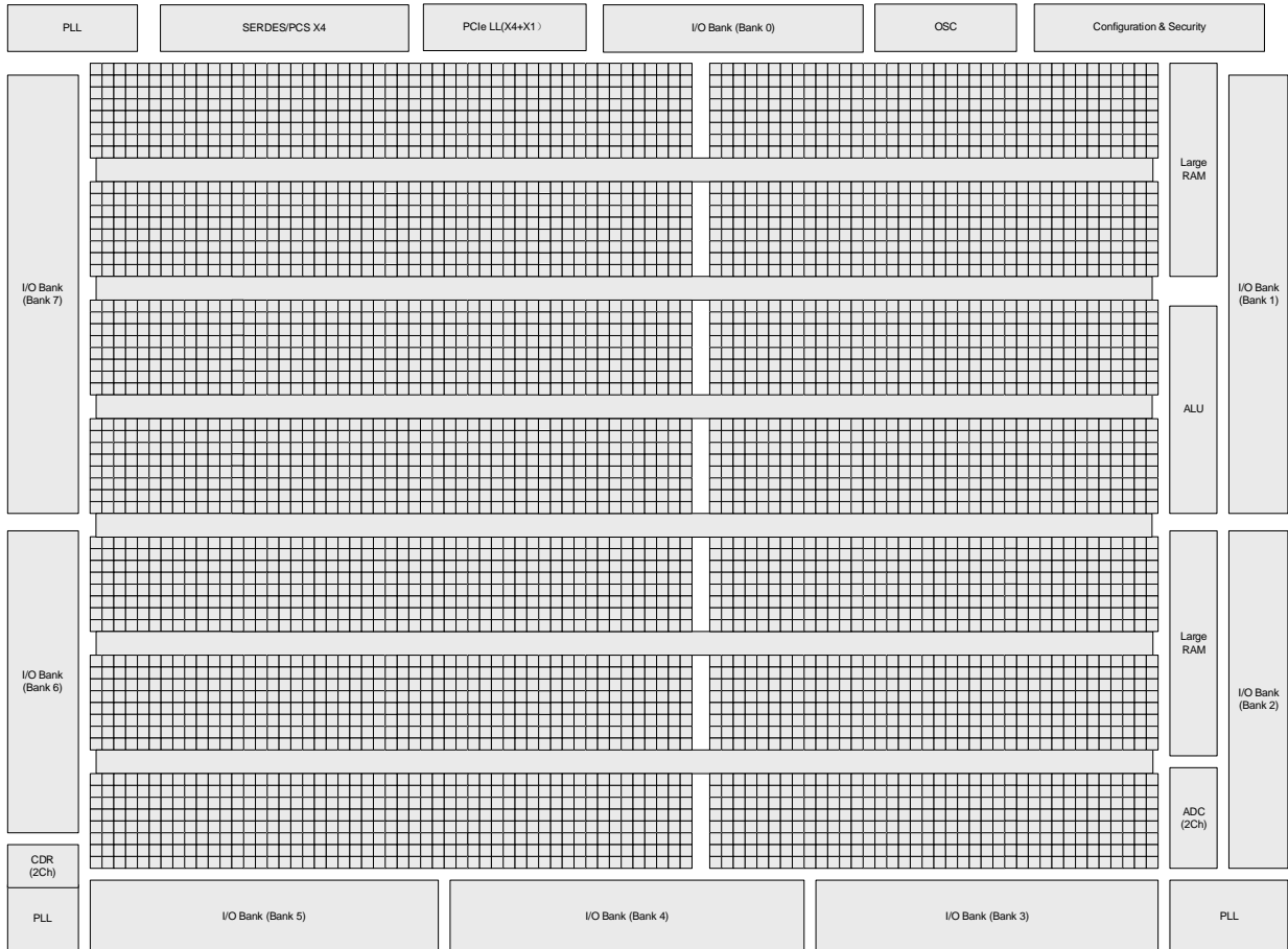
Figure 2.1. Simplified Block Diagram, LFCPNX-50 Device (Top Level)
