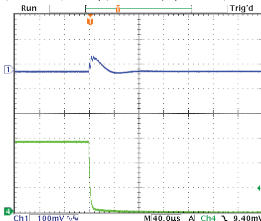
Step Load Transient Response (Vin=12V, Vout=5V, Cload=10x10µF X5R 0805 ceramic, plus 1x470µF, 7mΩ POSCAP, total 570µF, Iout=3A to 0A) Top trace=Vout, Bottom trace=Iout
