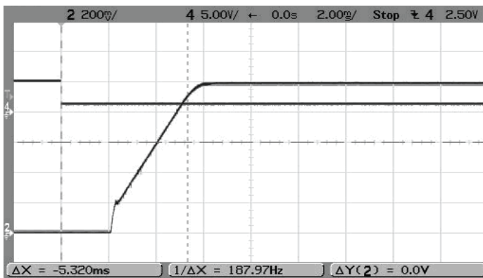
Step Load Transient Response (Vin = 5V, Vout = 1.0V, Cloud = 0, Iout = 1.5 to 3A) Trace 2 = Vout, 100 mV/div. Trace 4 = Iout, 2.5A/div.
