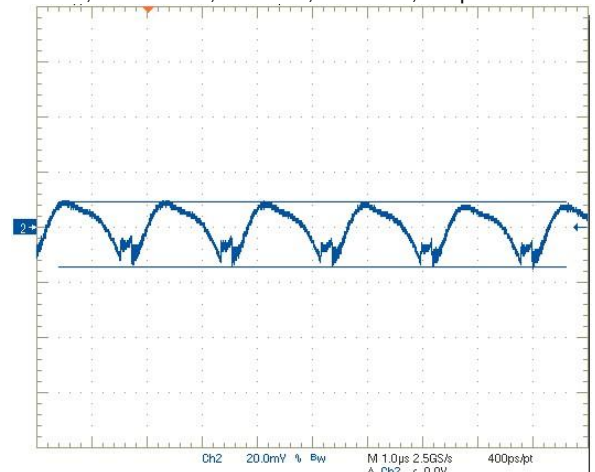
Step Load Transient Response (Vin = 12V, Vout = 1.2V, Clod = 0, Iout = 3 to 1.5A) Trace 2 = Vout, 100 mV/div. Trace 4 = Iout, 2.5A/div.
