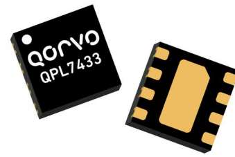
2X2 DFN 8pin Package
