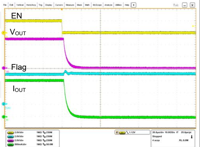
(VIN = 5 V, ROUT = 3.3 Ω, EN = 5 V ↓ 0)
