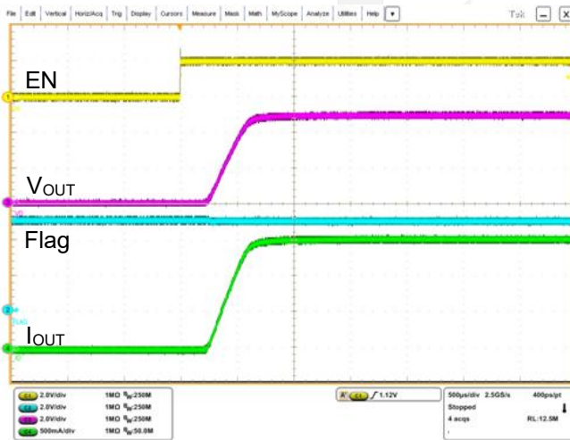
(VIN = 5 V, ROUT = 3.3 Ω, EN = 0 ↑ 5 V)
