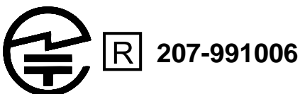
Figure 14: Giteki mark, and the EMMY-W163 MIC certification number. The "Indoor use only" information translated into Japanese below is mandatory if the product is operating in the 5.2/5.3 GHz band.
