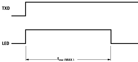
Figure 4. TXD "stuck on" protection waveform.
