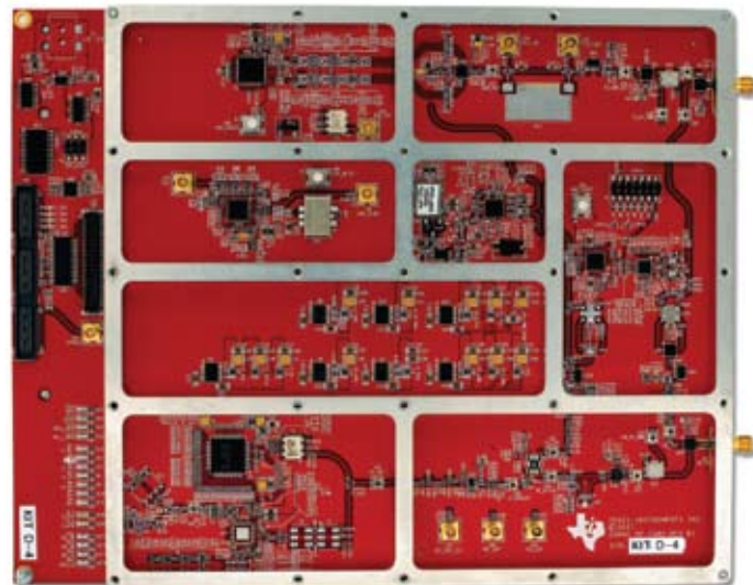
▲ GC5322SEK: 20-MHz Bandwidth RF Card
