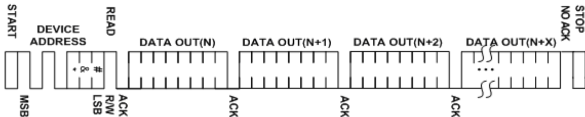
Figure 7: SEQUENTIAL READ (SDA INPUT/OUTPUT)
