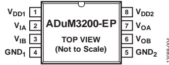
Figure 4. ADuM3200-EP Pin Configuration
