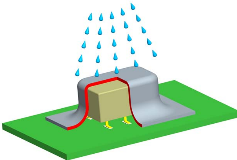
Fig. 11: Coating of relays on PCB's
