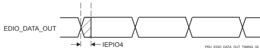
Figure 6-100. PRU_ICSSG IEP Digital IOs Timing Requirements
