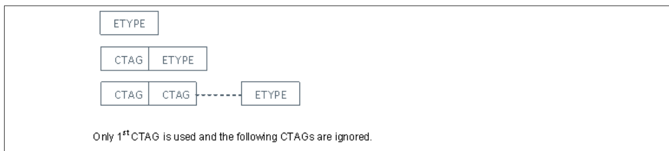
Figure 30 Supported Frame Formats when STAG is disabled
