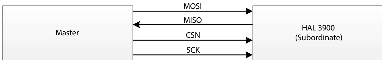
Fig. 3–16: Description of the SPI bus (example for HAL 3900)
