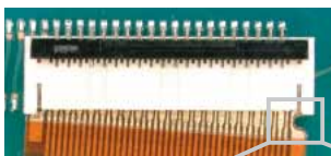
Incomplete FPC insertion
