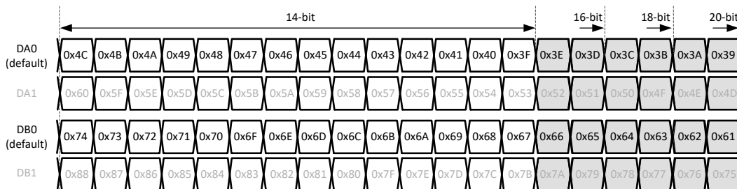
Figure 8-38. 1-wire output bit mapping
