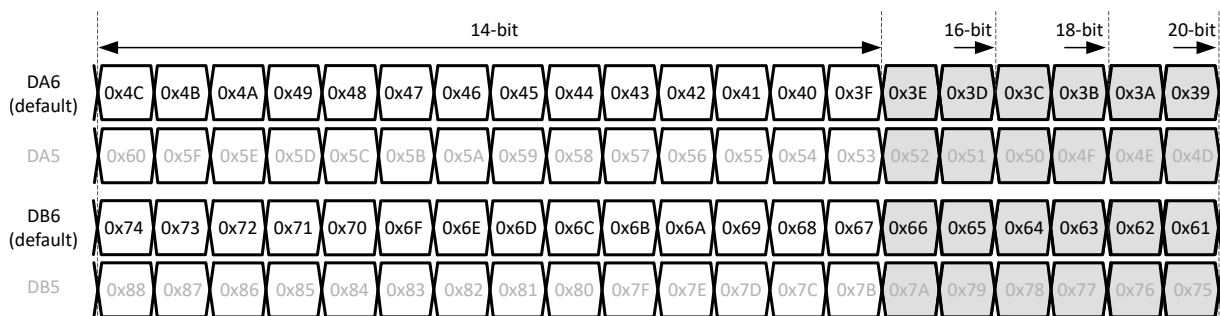
Figure 8-41. 1-wire output bit mapping
