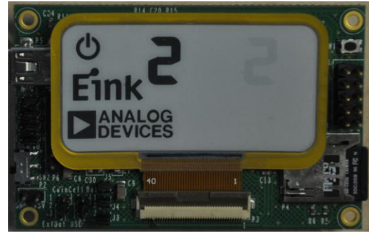
Figure 31. E-Ink Display for Second Inactivity Interrupt
