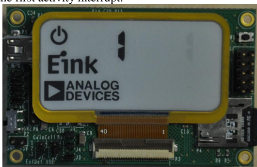
Figure 30. E-Ink Display for First Inactivity Interrupt
