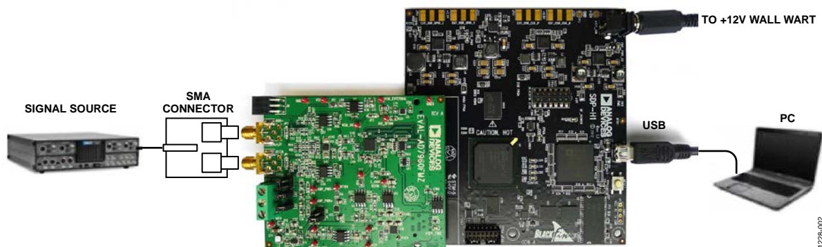
Figure 1. Setting Up the EVAL-AD7960FMCZ
