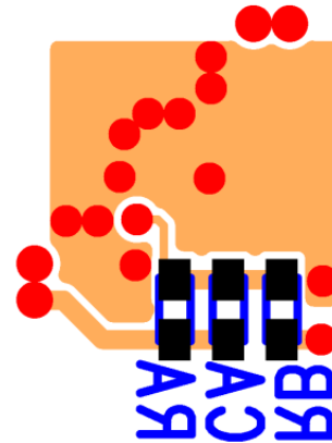
Figure 5: Bottom PCB Layer Critical Components ( R_A , R_B , C_A ) & Copper for Minimum Footprint
