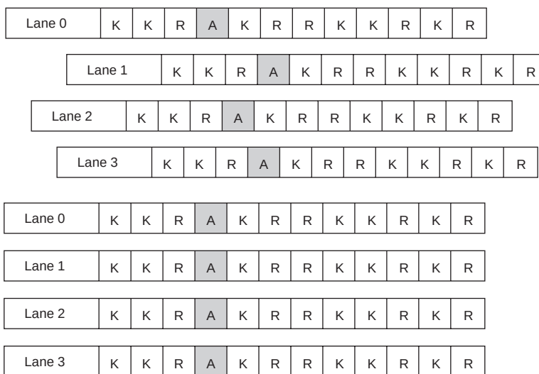
Figure 5-7. Example of Lane Skew at Receiver Input
