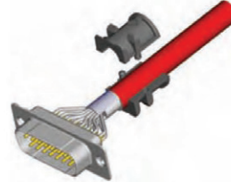
Attach the strain relief around the cable
