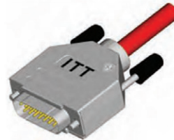
Assemble the other half (screwing force: 100-120 Ncm)
