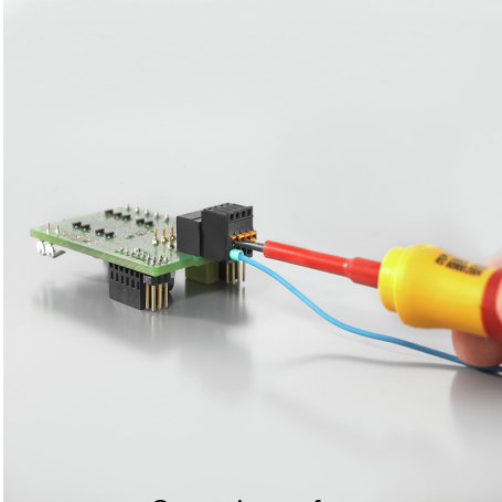
Operating safety Through PUSH IN connection system
