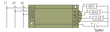
CR4850 3 Element, 3 Wire - 0 - 5 VDC Output CR4860 3 Element, 3 Wire - 4-20 mA DC Output
