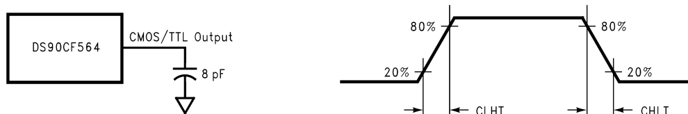
Figure 6. DS90CF564 (Receiver) CMOS/TTL Output Load and Transition Times
