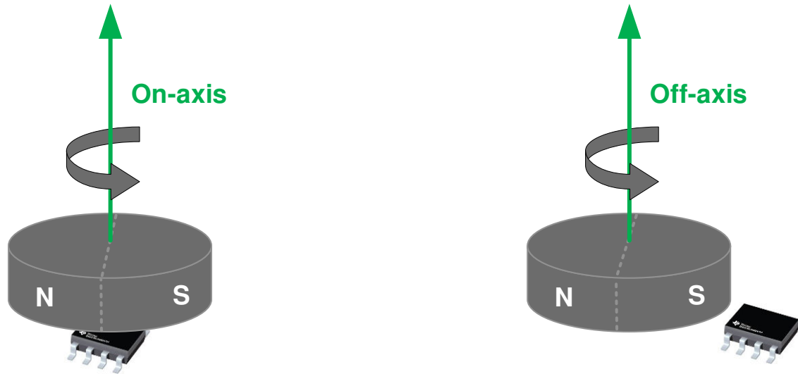
Figure 8-5. On-Axis vs. Off-Axis Angle Measurements
