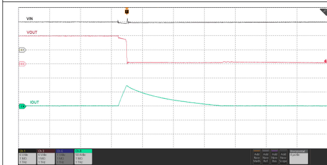
Figure 6-26. Inrush Current with Resistive and Capacitive Load
